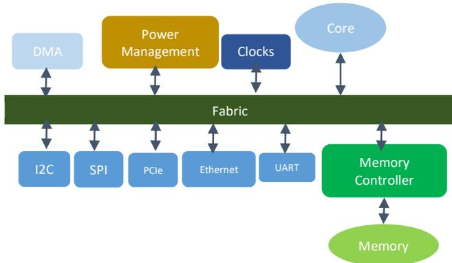
Fig. 1. A typical Microcontroller based Subsystem
