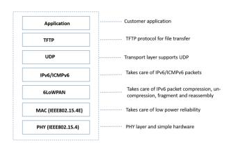
Fig. 5. RapidNet IP stack used by ESL network components
