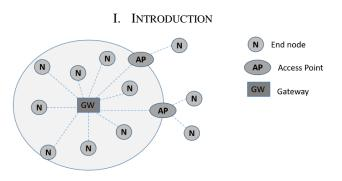
Fig. 1. RapidNet IP wireless network
