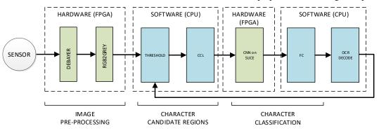
Fig. 3 Pipeline for OCR Accleration
