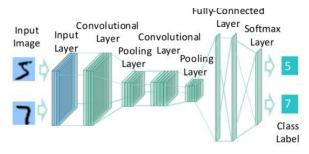
Fig. 2 CNN topology for OCR
