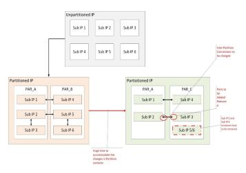
Fig. 2: Efforts needed for a simple change of partition contents
