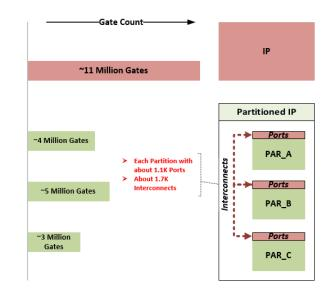
Fig. 1: Sample IP Partition complexity
